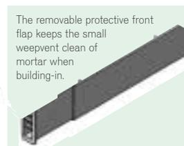
The removable protective front flap keeps the small weepvent clean of mortar when building-in.
